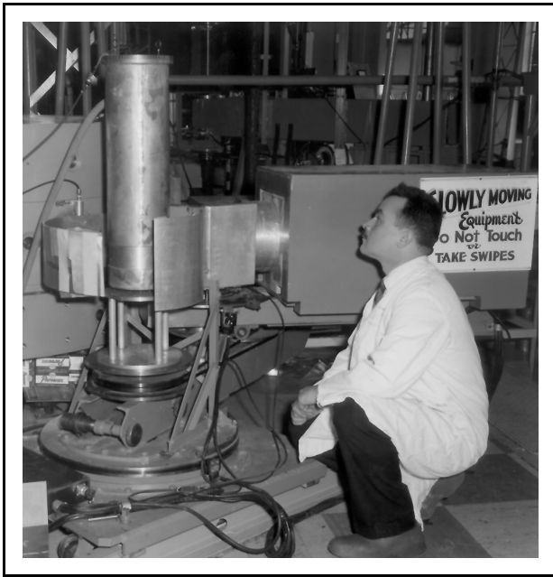
Fig. 1 Bert Brockhouse looking at the triple-axis spectrometer. The neutron beam comes from the left out of a large shielded drum containing the monochromator. The cryostat and analyser arm are carried on a Bofors gun mount driven by steel belts. To the right is the shielding around a long BF3 neutron detector. The “swipes” were taken not by frustrated physicists, but by health surveyors ensuring that the shield was clean.
